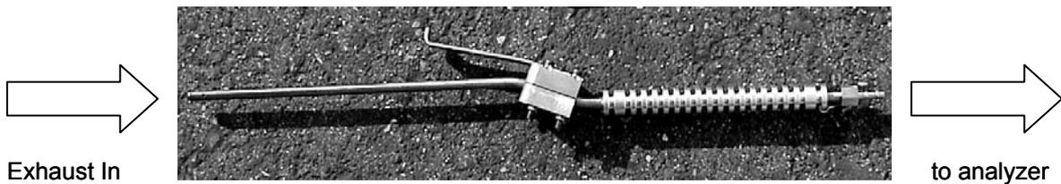
The exhaust probe which goes into the exhaust pipe has a length of 30 cm (left part of the probe). The tip of the probe is closed and has four small holes, drilled sideways into the probe. Normally, aircraft piston engines have rather short exhaust pipes. Therefore a cooling device as seen on the right hand side is necessary for cooling the exhaust gas in the probe from around 600°C to 200°C measuring temperature.
