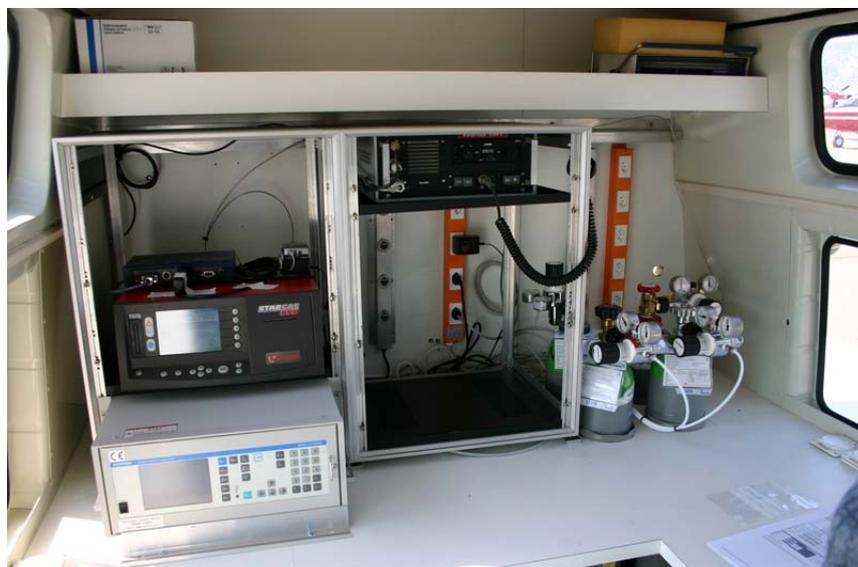
**f) Measurement systems for total HC measurements (certification standard)**
