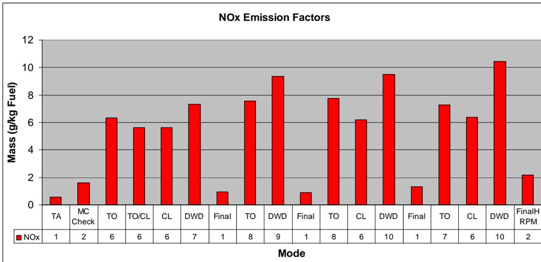
Figure 83: NO<sub>x</sub> emission factors during four aerodrome circuits (TA = Taxi, MC = Magneto Check, TO = Take off roll, CL = Climb at vy, DWD = downwind), flown at Samedan Airport (ECERT 59, HBKIA)
