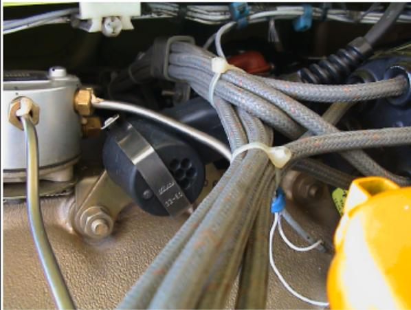
D) Installation of RPM sensor, overview
