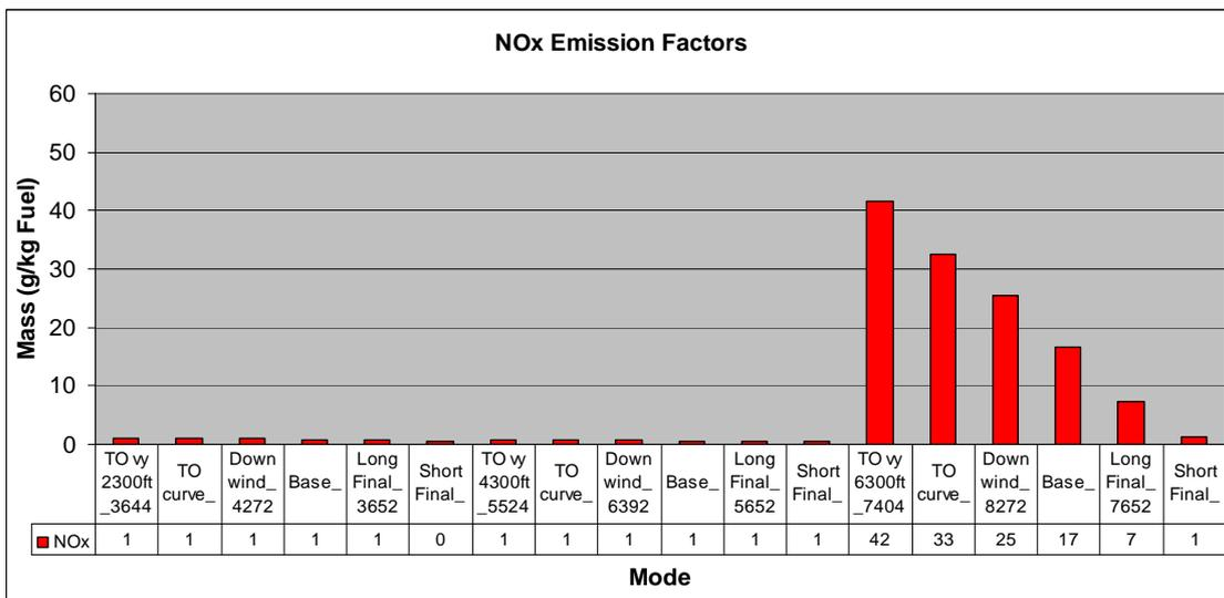
Figure 42: NO<sub>x</sub> emission factors in three simulated circuits, starting at 2300ft, 4300ft and 6300ft. The first two circuits were flown with air/fuel mixture “full rich”, the circuit above 6300ft with leaned mixture (right hand side). (ECERT22, HBKEZ)
