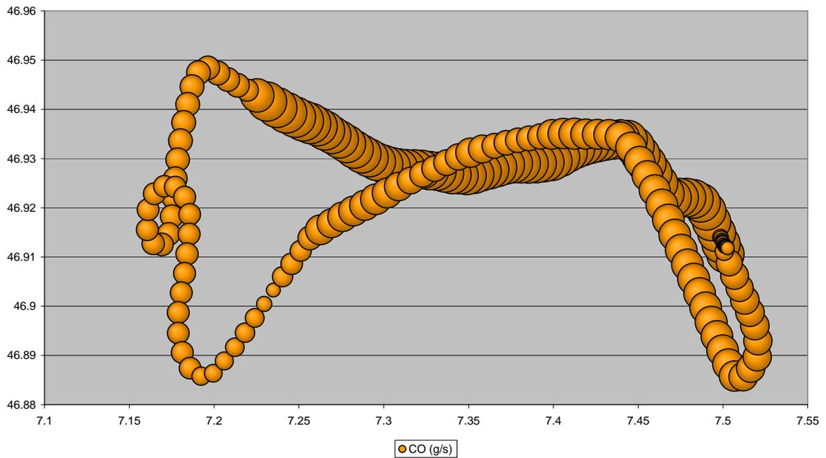
Figure 131: CO emissions during flight HBHFX 1537 (22.03.2006), the same flight as shown in figure 129 but without geographical background information. CO emissions are practically contrary to NO<sub>x</sub>: Very high during take-off and climb, lower during cruise and high during approach. The bubble size goes from around 9 to 70 (!) grams CO per 10 seconds.
