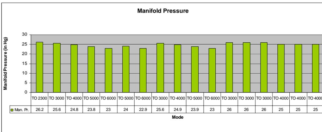
Figure 92: Manifold pressure for full power climb, measured at different flight altitudes, e.g. TO 2300 means take-off measurement at 2300ft pressure altitude (From left to right: No 1 – 7 from ECERT58, No 8 – 11 from ECERT61 and No 12 – 17 from ECERT65).
