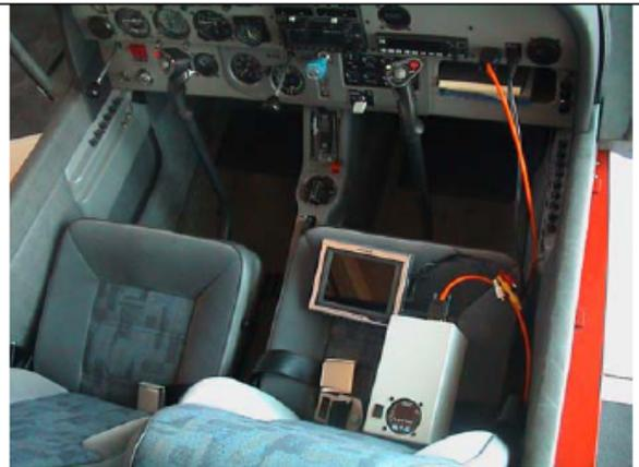
Exhaust tester: control monitor and fuel flow indicator. To control the air quality, a carbon monoxide detector, type Quantum Eye is installed in the cockpit.
