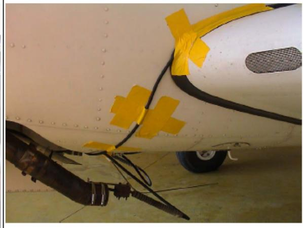
G) Exhaust probe and fixation (mounted with experience from HBEYS and HBKEZ in-flight testing). Flexible sampling line (Viton) with t-shape tube. First fixation point of sampling line is most important. In case, sampling line would disconnect or would be teared backwards, no obstruction of flight safety relevant parts has been found.
