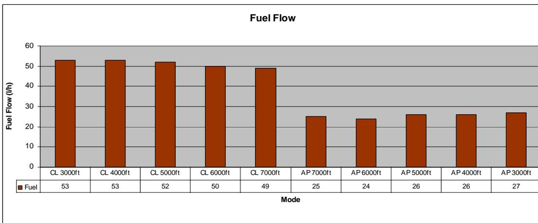
Figure 33: The fuel flow decreases with increasing height. During descent, the fuel flow has slightly increased (ECERT 11). Approach power has been higher at 3000ft than at 7000ft (see figure 34).
