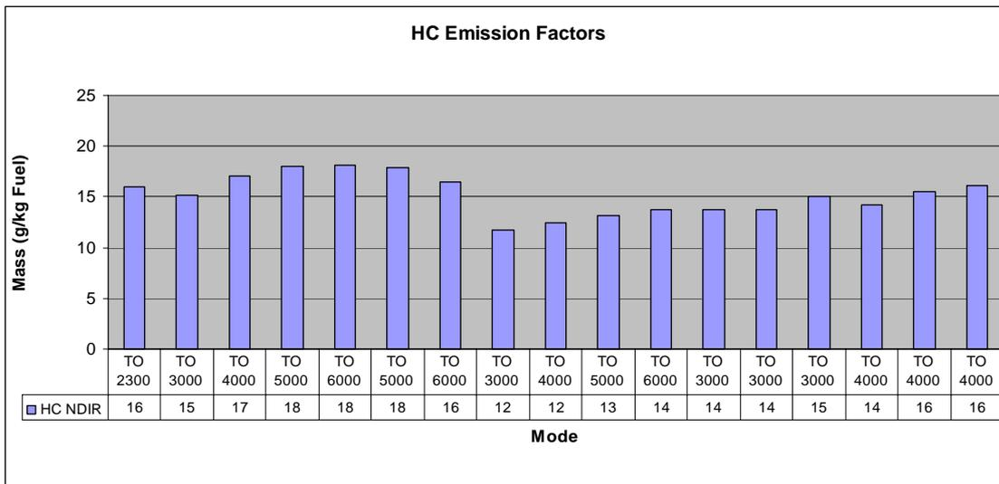
Figure 88: HC emission factors for full power climb, measured at different flight altitudes, e.g. TO 2300 means take-off measurement at 2300ft pressure altitude (From left to right: No 1 – 7 from ECERT58, No 8 – 11 from ECERT61 and No 12 – 17 from ECERT 65).
