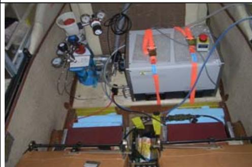
Installation of the on board measurement system. The fixation is done with two clamps which are passing underneath the wooden board. The gas bottles (synth. air and He/H<sub>2</sub>) are fixed with 4 clamps to the metallic support. The pipe for He/H<sub>2</sub> is made out of stainless steel with a reserve length of 1 m. The various links on the gas lines are tested with special gas leakage spray. A pressure drop during measurement would be signalled by the system.
