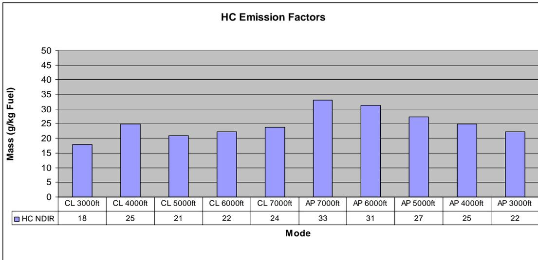
Figure 31: Effect on HC emission factor. At approach power, HC emission factors are higher than at climb power (ECERT 11). During descent, approach power has been slightly increased above 45% engine load, compared to ECERT 8 (figure 25). In spite of that, HC emission factors for approach show similar values between 22 and 33 g/kg fuel.
