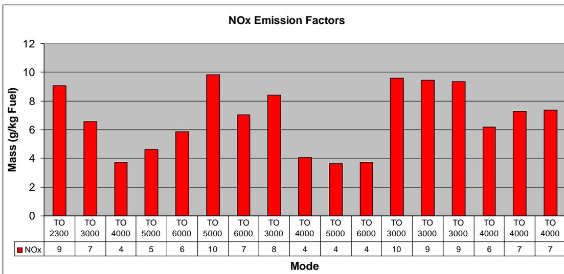
Figure 89: NO<sub>x</sub> emission factors for full power climb, measured at different flight altitudes, e.g. TO 2300 means take-off measurement at 2300ft pressure altitude (From left to right: No 1 – 7 from ECERT58, No 8 – 11 from ECERT61 and No 12 – 17 from ECERT 65).
