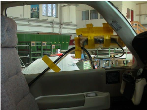
L) Sampling line guidance along airframe near flap section. Even loose flexible sampling line can not obstruct flap operation.
