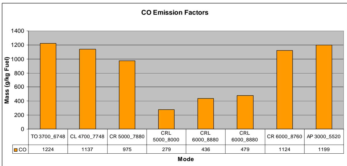
Figure 1: CO emission factors for take-off, climb, cruise and approach. TO, CL, CR5000\_7748, CR6000\_8760 and AP have been flown with air-fuel mixture “full rich”. CRL has been flown with manually adjusted engine air-fuel mixture.
