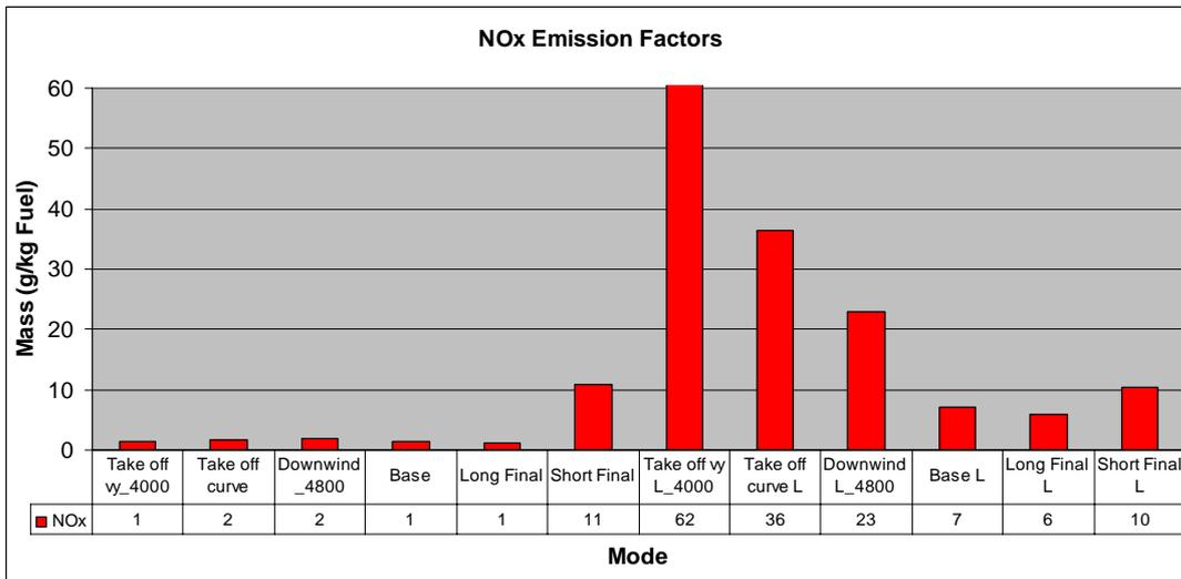
Figure 11: NO<sub>x</sub> emission factors during two aerodrome circuits, starting at 4000ft, downwind at 4800ft. The second circuit has been flown with leaned mixture as described in 1.c. (ECERT 4.2, HBEYS)
