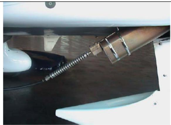
Probe set on exhaust pipe
