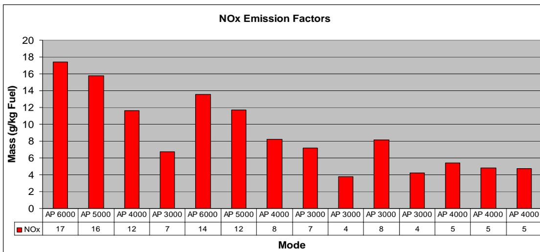
Figure 103: NO<sub>x</sub> emission factors for approach power, measured at different flight altitudes, e.g. AP 6000 means approach measurement at 6000ft pressure altitude (From left to right: No 1 – 7 from ECERT58, No 8 – 11 from ECERT61 and No 12 – 17 from ECERT 65).
