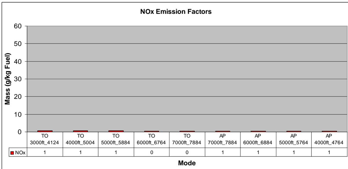
Figure 47: NO<sub>x</sub> emission factors during climb at full power (TO) from 3000 to 7000ft and during descent from 7000 to 3000ft (AP). With the very rich mixture, practically no NO<sub>x</sub> is built up. (ECERT27, HBKEZ)
