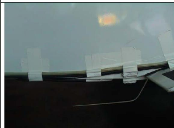
Exhaust line: along fuselage
