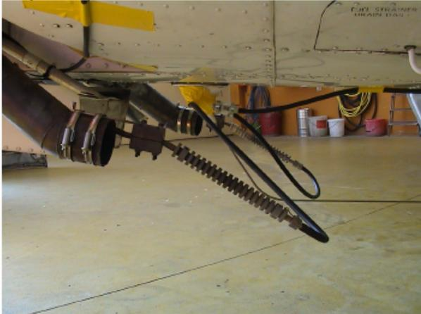
H) Fixation of exhaust in – and out lines on left hand fuselage. Tape placing with experience from HBEYS and KEZ testing. HBKEZ has been operated up to 130 kn without tape becoming loose.
