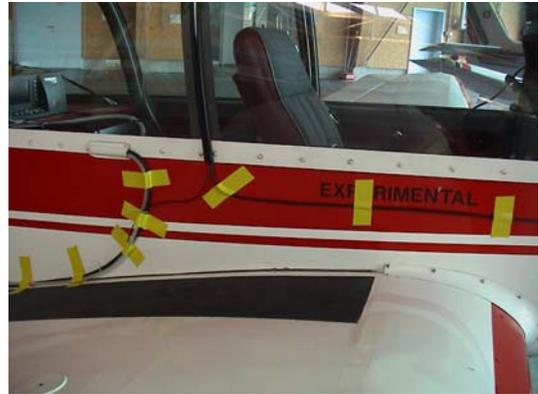
Picture 2: Sampling lines in and out
