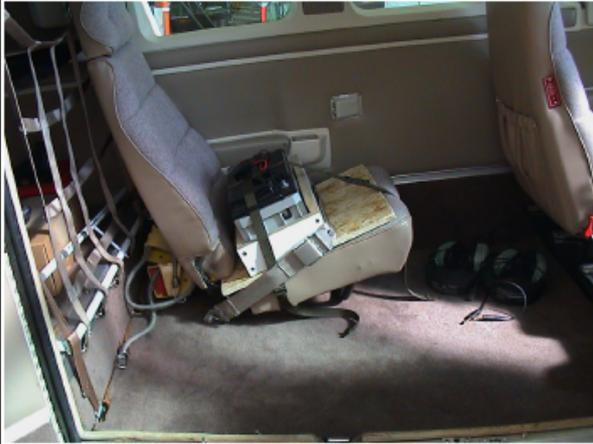
B) Installation of Stargas898 unit (total Mass 10 kg)
