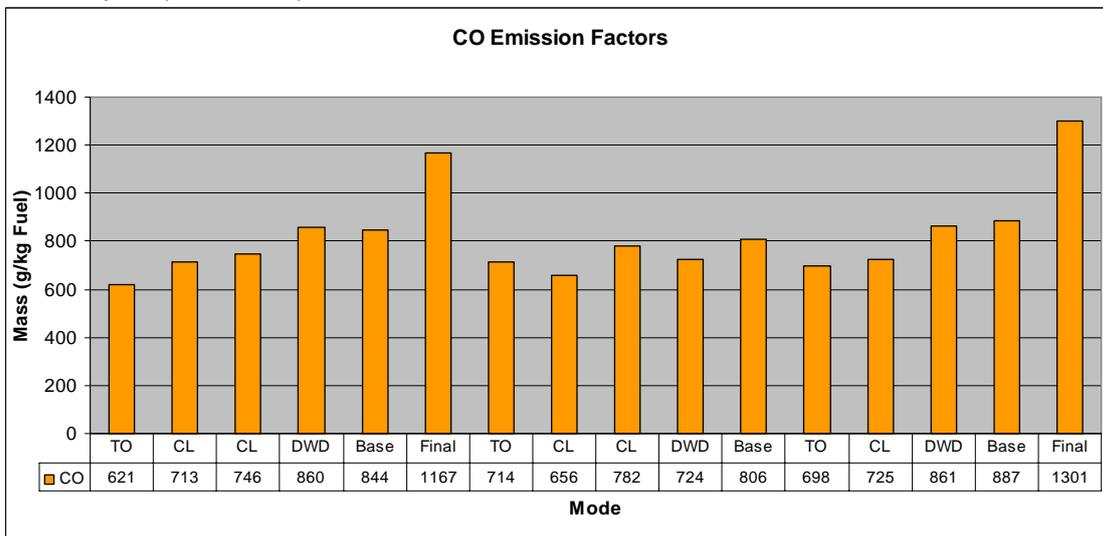
Figure 69: CO emission factors during three aerodrome circuits (TO = Take off roll, CL = Climb at  $v_y^5$ , DWD = downwind). No "Final" measurement at the second circuit. (ECERT 56, HBKIA)
