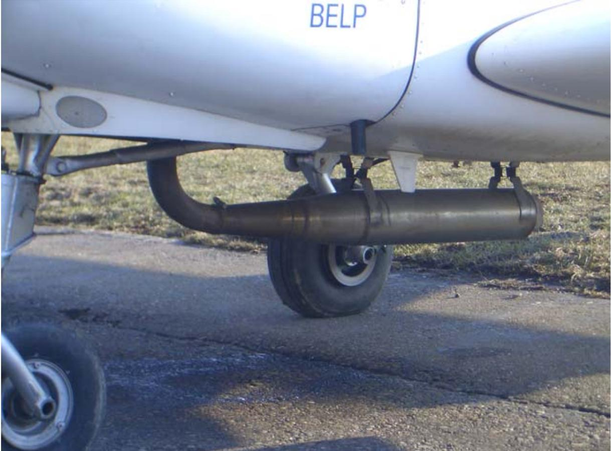
Picture 8: HB-HFX with original exhaust muffler (Gomolzig).
