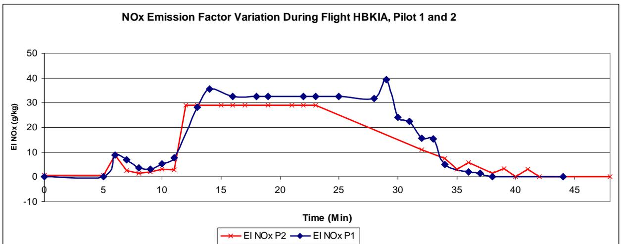
Figure 124: Comparison of NO<sub>x</sub> emission factor variation during flights with pilot 1 and 2. Please note, that the decrease of EI NO<sub>x</sub> P2 (pilot 2) between 23 and 32 minutes after off-block is artificial, because of missing data points, as in figure 122.
