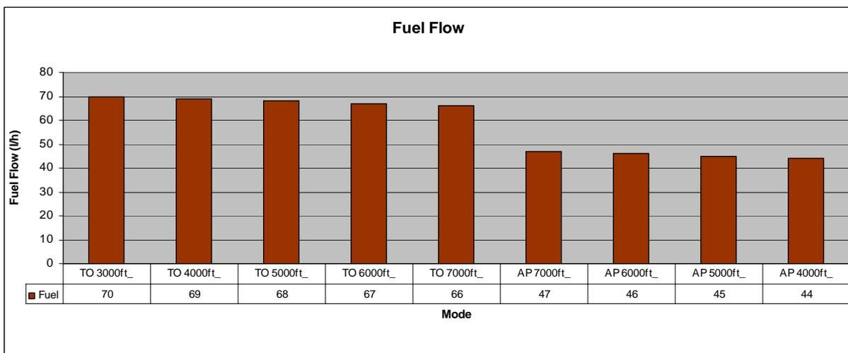
Figure 48: Fuel flow during climb at full power (TO) from 3000 to 7000ft and during descent from 7000 to 3000ft (AP). (ECERT27, HBKEZ)
