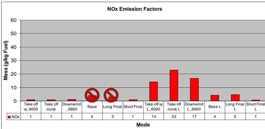
Figure 12: NO<sub>x</sub> emission factors during two aerodrome circuits, starting at 6000ft, downwind at 6800ft. The second circuit has been flown with leaned mixture as described in 1.c. (ECERT 4.3, HBEYS). The first base leg was measured during power adjustments and is not considered valid.
