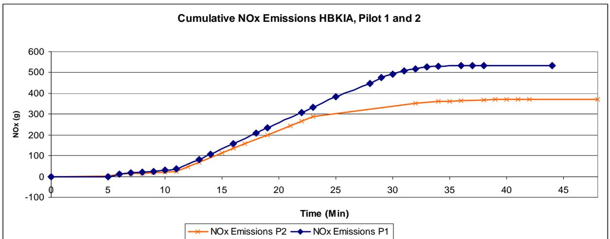
Figure 128: Comparison of cumulative NO<sub>x</sub> emissions during flight with pilot 1 and 2. In this example, the lower power setting during cruise and descent, chosen by pilot 2 results in lower NO<sub>x</sub> emissions. The highest portion of NO<sub>x</sub> emissions occurs during cruise.
