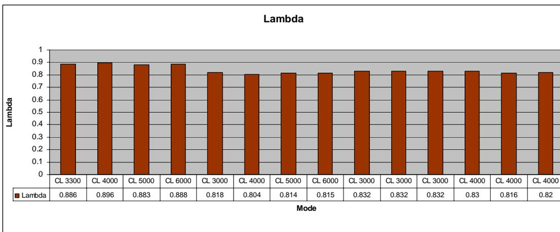
Figure 100: Lambda for AFM climb power, measured at different flight altitudes, e.g. CL 3300 means climb measurement at 3300ft pressure altitude (From left to right: No 1 – 7 from ECERT58, No 8 – 11 from ECERT61 and No 12 – 17 from ECERT 65).
