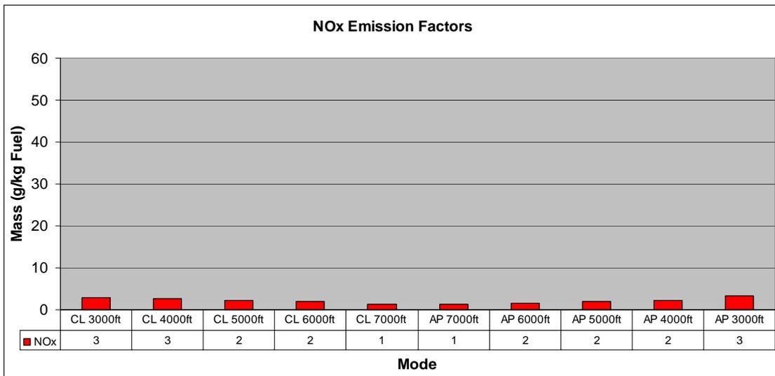
Figure 32: NO<sub>x</sub> emission factors are very low and comparable to figure 26 due to low internal combustion temperatures. With increasing height, the NO<sub>x</sub> emission factor decreases (without mixture adjustment). (ECERT 11)
