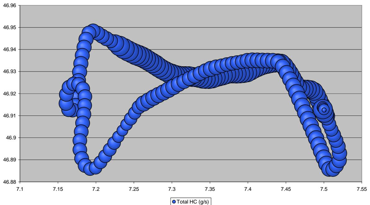
Figure 132: Total HC emissions during flight HBHFX 1537 (22.03.2006), the same flight as shown in figure 129 but without geographical background information. HC emissions are particularly high during take-off and climb, lower during cruise and higher during approach. The bubble size goes from around 0.4 to 1.2 grams HC per 10 seconds.
