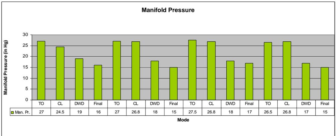
Figure 79: Manifold pressure during four aerodrome circuits (TO = Take off roll, CL = Climb at v<sub>y</sub>, DWD = downwind), flown with second pilot (ECERT 62, HBKIA)
