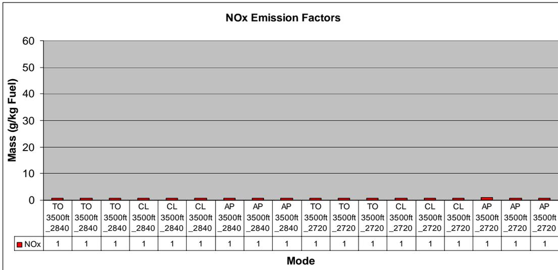
Figure 52: NO<sub>x</sub> emission factors during take-off, climb and approach, when passing 3500ft (2800ft density altitude.) Two flights at different days. (ECERT48+49, HBKEZ)
