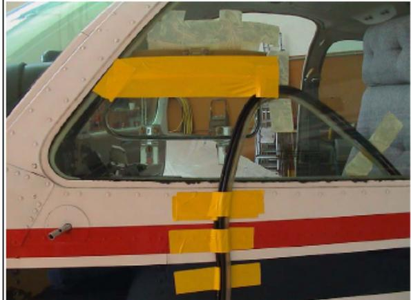
K) Sampling line guidance from inside. Reduced visibility to left hand side for the PIC has to be taken into account during in-flight tests. -> AFM supplement.
