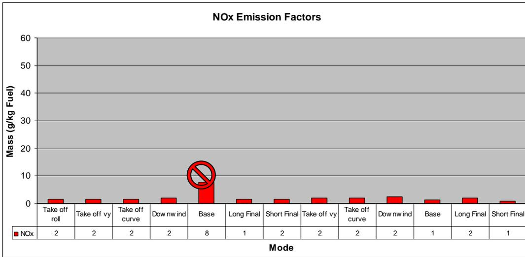
Figure 10: NO<sub>x</sub> emission factors during two aerodrome circuits, starting at 2000ft, downwind at 2800ft. (ECERT 4, HBEYS). The first base leg was measured during power adjustments and is not considered valid.
