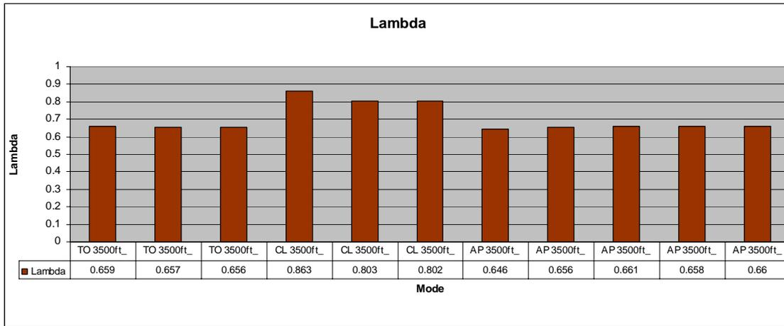
Figure 60: Lambda values: The leaning procedure in climb according AFM leads to lambda values around 0.85 (ECERT 47, HBKEZ).
