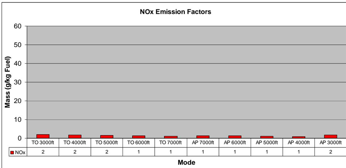
Figure 26: NO<sub>x</sub> emission factors are very low due to low internal combustion temperatures. With increasing height, the NO<sub>x</sub> emission factor decreases (no mixture adjustment). (ECERT 8)
