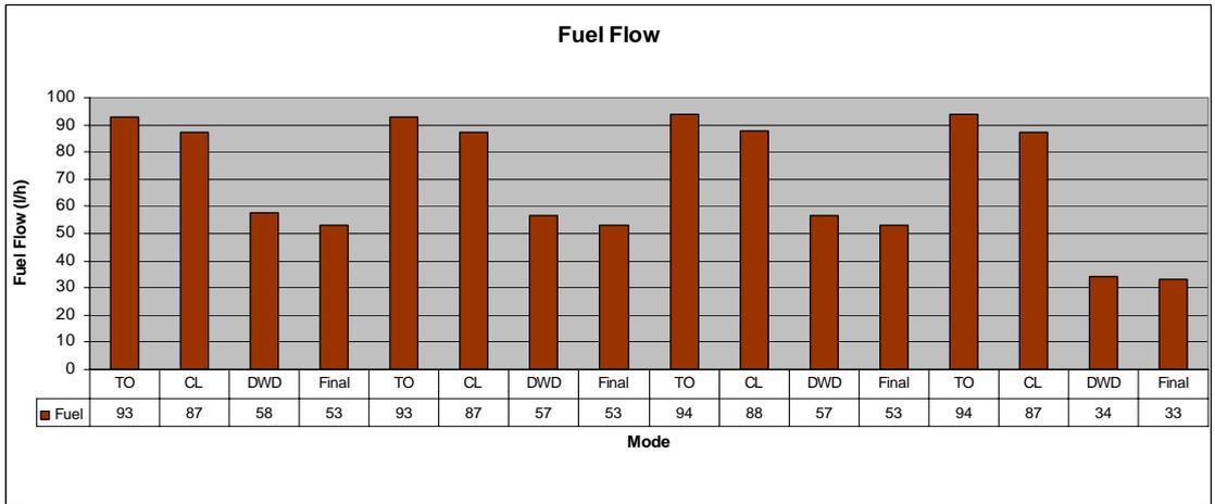
Figure 78: Fuel flow during four aerodrome circuits (TO = Take off roll, CL = Climb at v<sub>y</sub>, DWD = downwind), flown with second pilot (ECERT 62, HBKIA)
