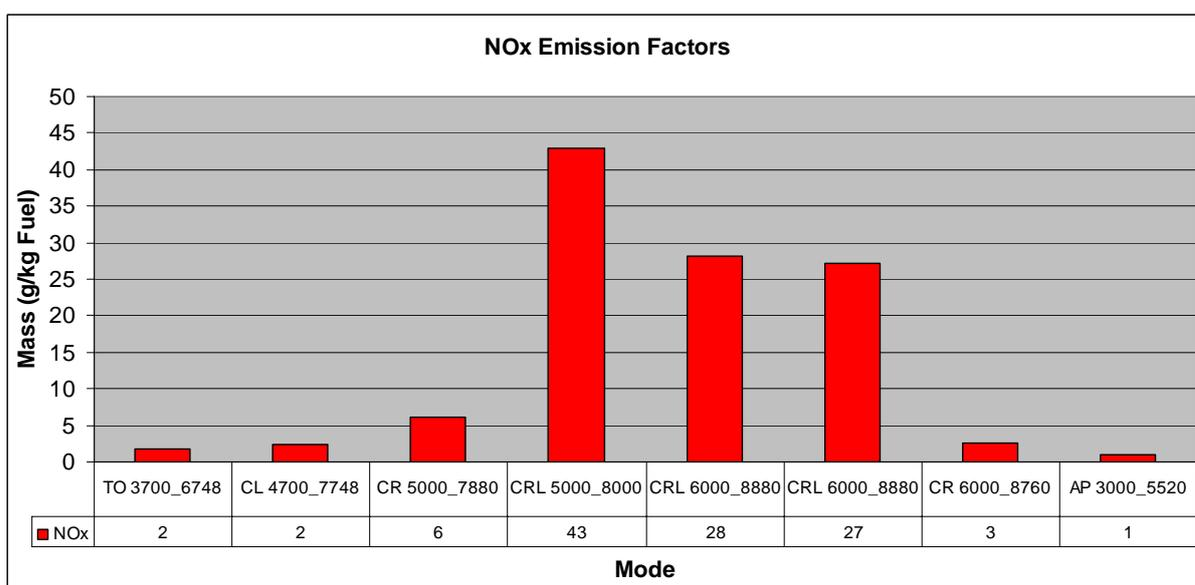
Figure 3: NO<sub>x</sub> emission factors for take-off, climb, cruise and approach. TO, CL, CR5000\_7748, CR6000\_8760 and AP have been flown with air-fuel mixture “full rich”. CRL has been flown with manually adjusted air-fuel mixture.
