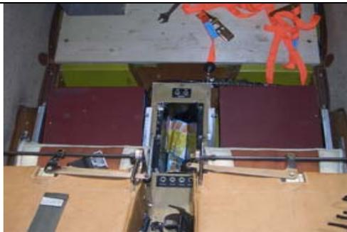
Batteries are mounted. Any possible upward movement of the batteries is prevented by the front seats once these are back in place.
