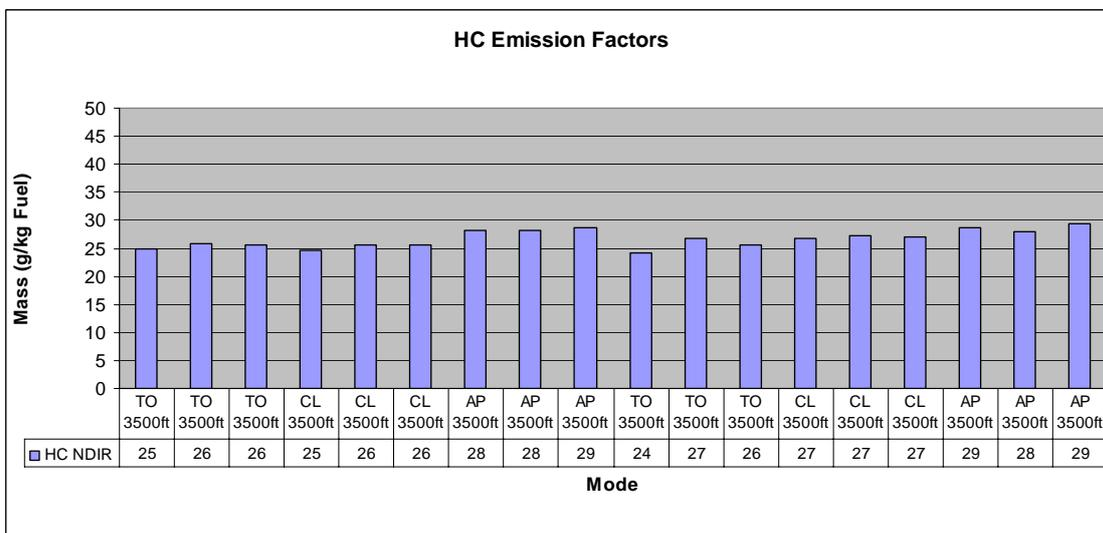
Figure 51: HC emission factors during take-off, climb and approach, when passing 3500ft (2800ft density altitude.) Two flights at different days. (ECERT48+49, HBKEZ)
