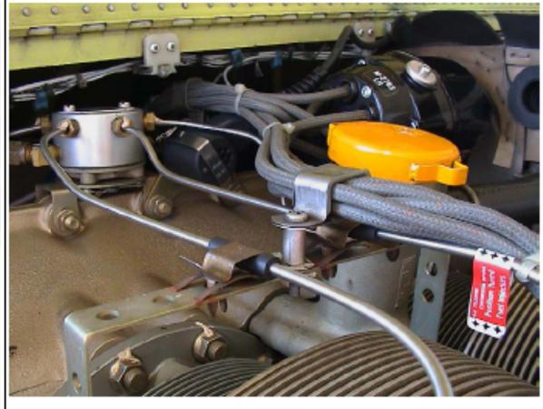
E) RPM sensor signal line (black, from left top to right bottom)
