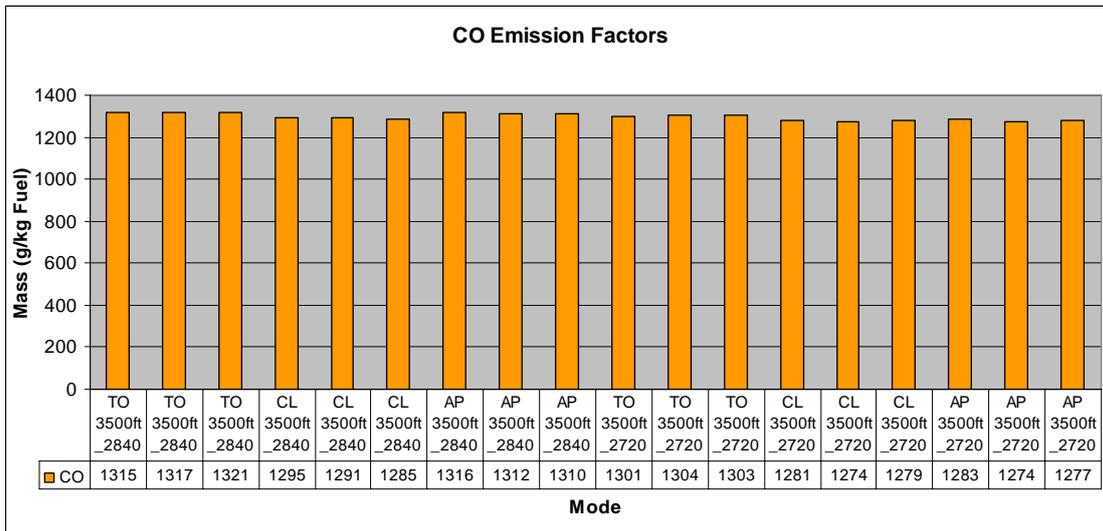
Figure 50: CO emission factors during take-off, climb and approach, when passing 3500ft (2800ft density altitude.) Two flights at different days. (ECERT48+49, HBKEZ)
