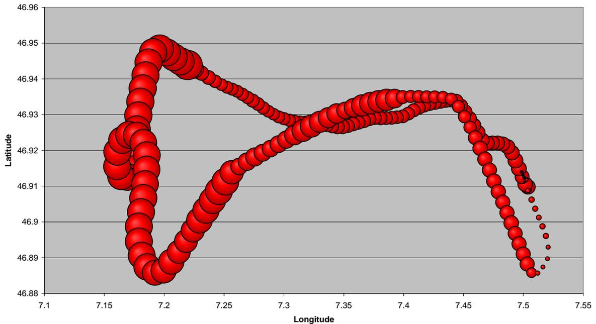
Figure 130: NO<sub>x</sub> emissions during flight HBHFX 1537 (22.03.2006), the same flight as shown in figure 129 but without geographical background information. With this illustration (“NO<sub>x</sub> worm”) the variation of NO<sub>x</sub> mass emissions during the flight can be seen very clearly. One “bubble” contains the NO<sub>x</sub> emissions integrated over 10 seconds flight time. The bubble size goes from around 0.05 to 2 grams NO<sub>x</sub> per 10 seconds.
