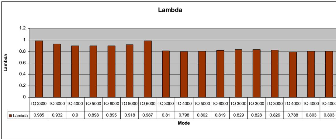
Figure 93: Lambda for full power climb, measured at different flight altitudes, e.g. TO 2300 means take-off measurement at 2300ft pressure altitude (From left to right: No 1 – 7 from ECERT58, No 8 – 11 from ECERT61 and No 12 – 17 from ECERT65).
