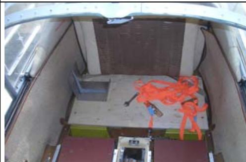
The back seat was taken off and a 2 cm thick wooden board was fixed on the fuselage. On the left side is the metallic support for the two little gas bottles.
