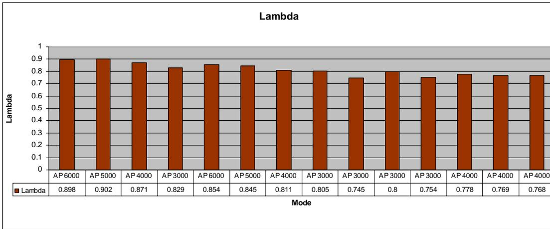
Figure 107: Lambda for approach power, measured at different flight altitudes, e.g. AP 6000 means approach measurement at 6000ft pressure altitude (From left to right: No 1 – 7 from ECERT58, No 8 – 11 from ECERT61 and No 12 – 17 from ECERT 65).
