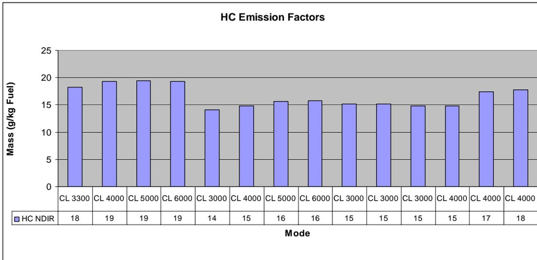
Figure 95: HC emission factors for AFM climb power, measured at different flight altitudes, e.g. CL 3300 means climb measurement at 3300ft pressure altitude (From left to right: No 1 – 7 from ECERT58, No 8 – 11 from ECERT61 and No 12 – 17 from ECERT 65).
