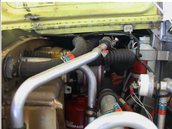
F) RPM signal line and exhaust probes
