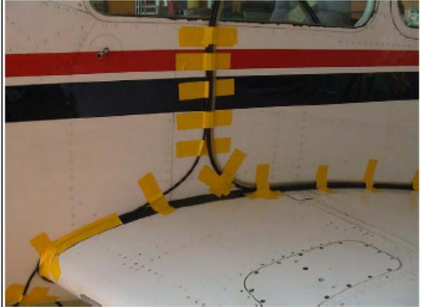
I) First fixation point of flexible sampling line from below.
