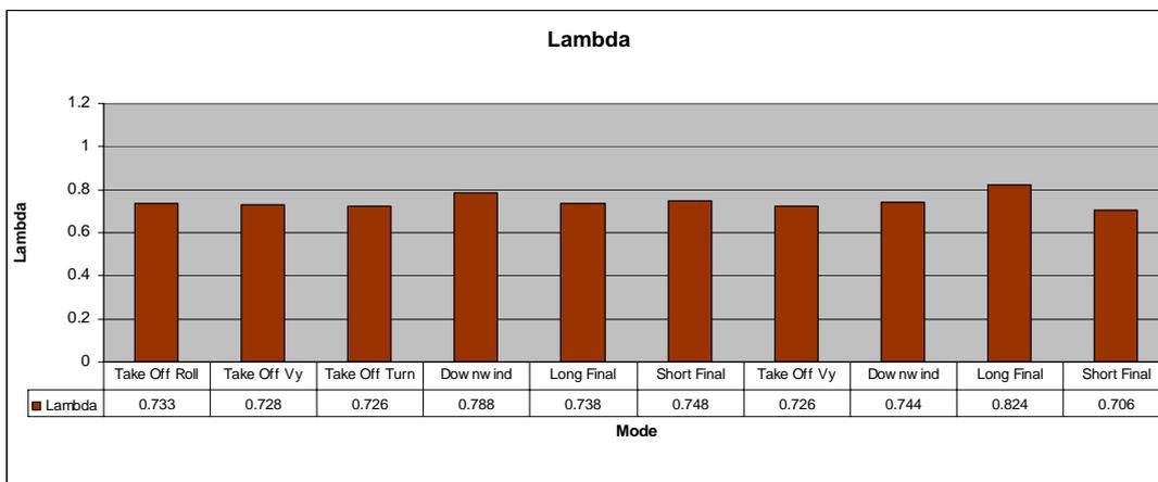
Figure 22: Lambda, measured during two circuits, starting at 5600ft, downwind at 6600ft. (ECERT 13)
