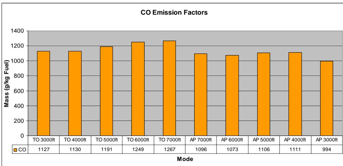
Figure 24: Effect on CO emission factor. With increasing height, the CO emission factor gets even worse (without mixture adjustment). (ECERT 8)
