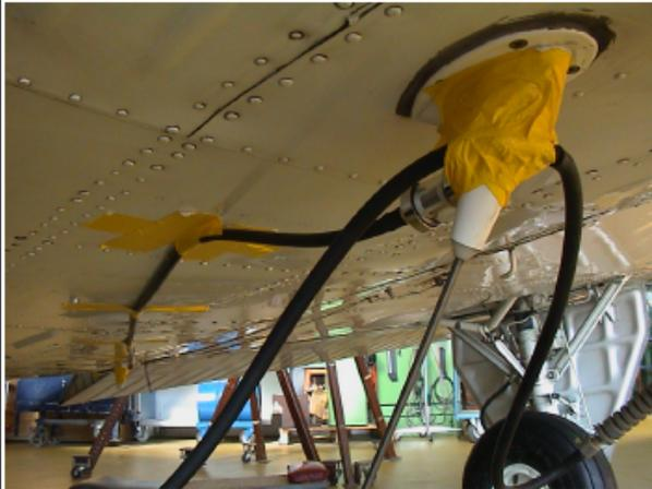
J) Guiding of exhaust sampling lines through side window. Window opening angle is defined by piece of foam.
