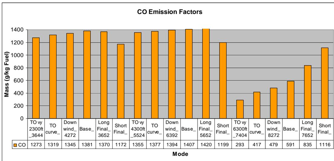
Figure 40: Record braking CO emission factors in three simulated circuits, starting at 2300ft, 4300ft and 6300ft. The first two circuits were flown with air/fuel mixture “full rich”, the circuit above 6300ft with leaned mixture (right hand side). (ECERT22, HBKEZ)
