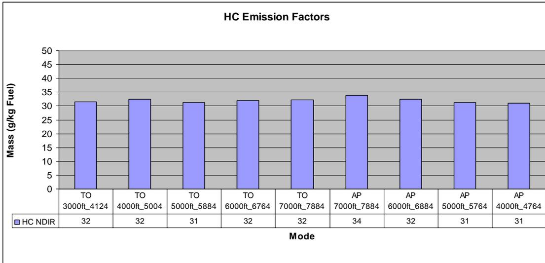
Figure 46: HC emission factors during climb at full power (TO) from 3000 to 7000ft and during descent from 7000 to 3000ft (AP). With the very rich mixture, they vary around 32 g / kg fuel. (ECERT27, HBKEZ)
