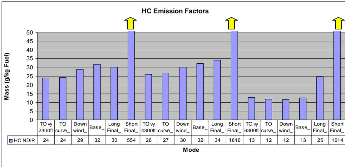
Figure 41: HC emission factors in three simulated circuits, starting at 2300ft, 4300ft and 6300ft. The first two circuits were flown with air/fuel mixture “full rich”, the circuit above 6300ft with leaned mixture (right hand side). Again, the same effect at engine idle, described in sections 3.c/d) can be seen. (ECERT22, HBKEZ)
