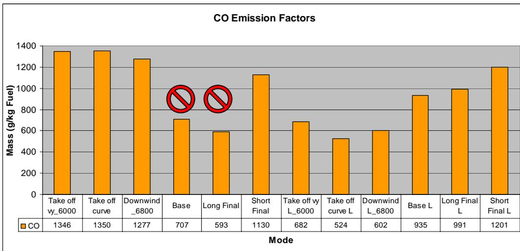
Figure 6: CO emission factors during two aerodrome circuits, starting at 6000ft, downwind at 6800ft. The second circuit has been flown with leaned mixture as described in 1.c. (ECERT 4.3 HBEYS) The first base leg was measured during power adjustments and is not considered valid.
