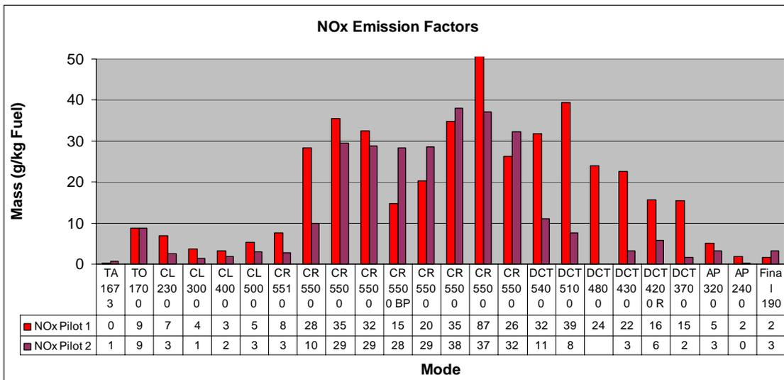
Figure 110: NO<sub>x</sub> emission factors comparison for both flights. TA = taxi, TO = take-off roll, CL = climb, CR = cruise, DCT = descent, AP = approach. The number below the flight mode indicates flight pressure altitude, e.g. DCT 5100 = measurement during descent at 5100ft. (ECERT 57 and 64)
