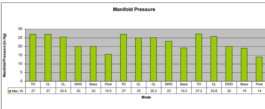
Figure 73: Manifold pressure during three aerodrome circuits (TO = Take off roll, CL = Climb at v<sub>y</sub>, DWD = downwind). No “Final” measurement at the second circuit. (ECERT 56, HBKIA)
