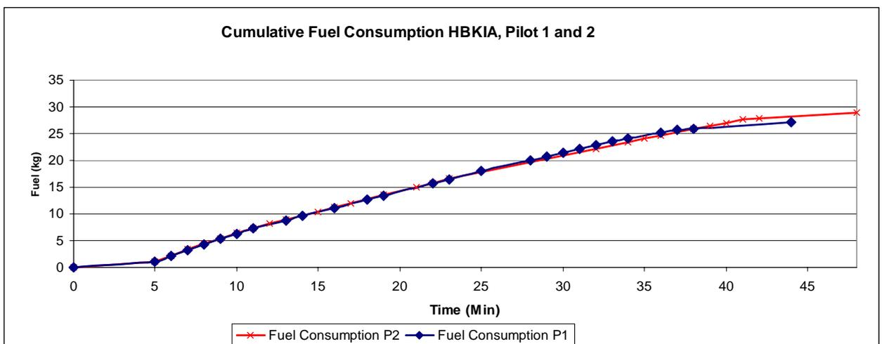
Figure 125: Comparison of cumulative fuel consumption during flight with pilot 1 and 2. In this example, pilot 2 chooses reduced cruise power. Hence the flight time is longer. Together with a suboptimal approach pattern, this adds up to higher total fuel consumption.
