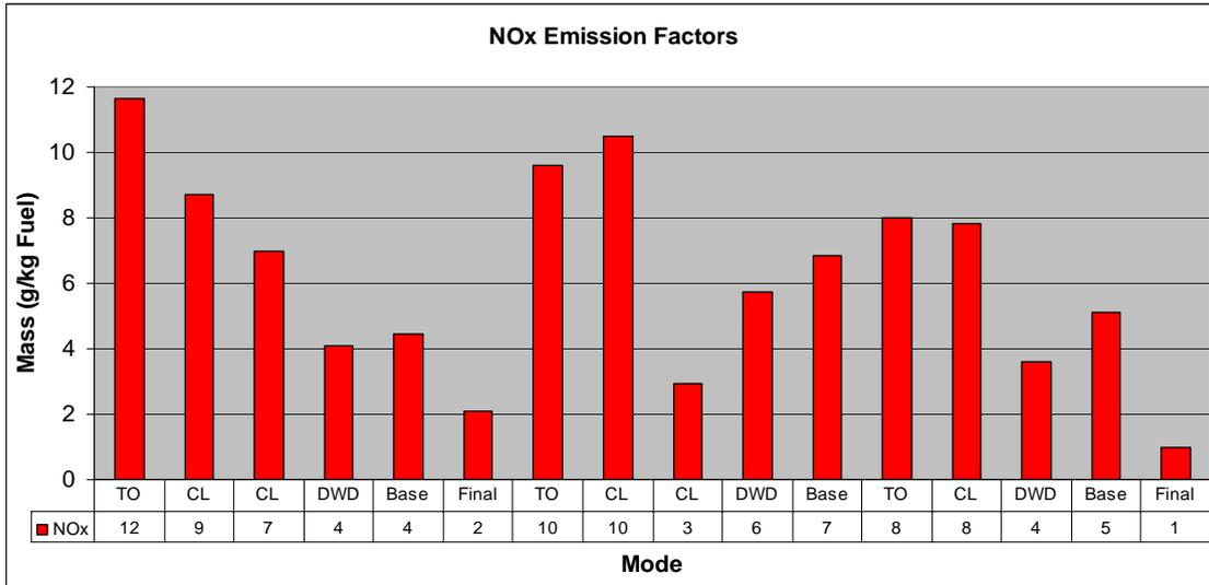
Figure 71: NO<sub>x</sub> emission factors during three aerodrome circuits (TO = Take off roll, CL = Climb at v<sub>y</sub>, DWD = downwind). No “Final” measurement at the second circuit. (ECERT 56, HBKIA)
