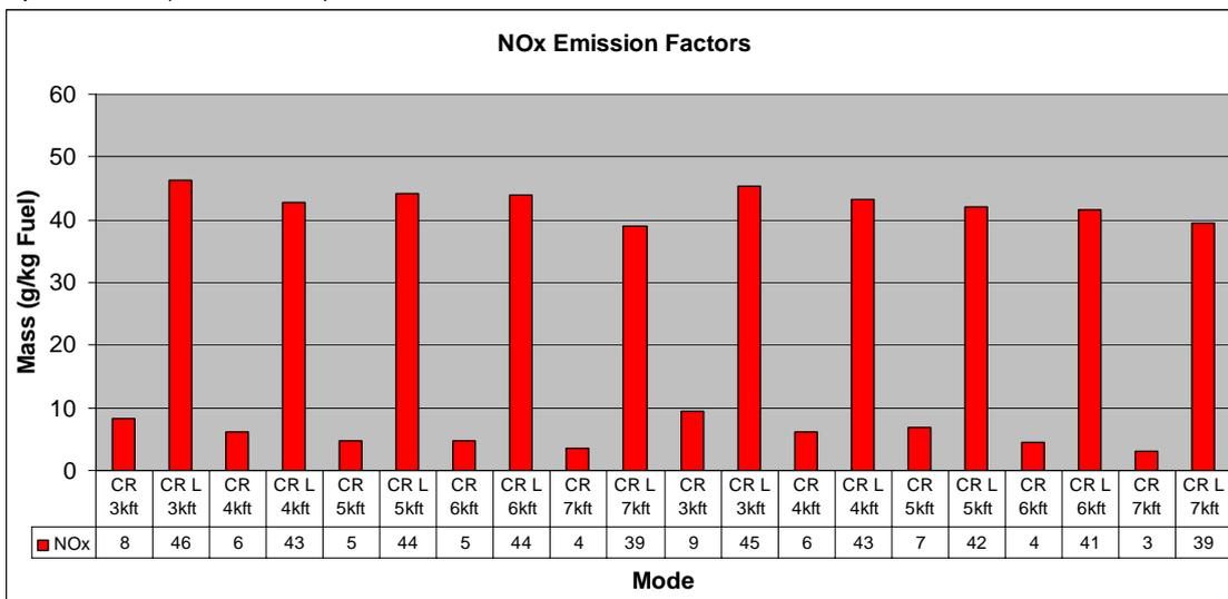
Figure 39: NO<sub>x</sub> emission factors decreasing with altitude without mixture adjustment. At stoichiometric mixture, the values get high (trade off with CO and HC) and are around 42 g / kg fuel. In terms of typical emission measurement accuracies, the values are considered reproducible. (ECERT 9/10)
