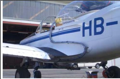
Collector pipe is fixed with choke collars directly screwed on the fuselage. The turbulences created by the collector pipe were investigated during the rolling test on runway in LSZB and did not interfere with the controls. In emergency, the canopy can be slide backward without hindrance.
