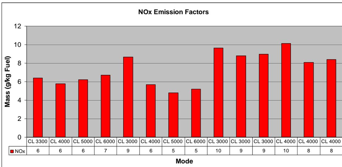
Figure 96: NO<sub>x</sub> emission factors for AFM climb power, measured at different flight altitudes, e.g. CL 3300 means climb measurement at 3300ft pressure altitude (From left to right: No 1 – 7 from ECERT58, No 8 – 11 from ECERT61 and No 12 – 17 from ECERT 65).
