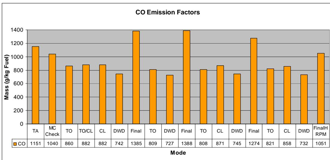
Figure 81: CO emission factors during four aerodrome circuits (TA = Taxi, MC = Magneto Check, TO = Take off roll, CL = Climb at vy<sup>7</sup>, DWD = downwind), flown at Samedan Airport (ECERT 59, HBKIA)
