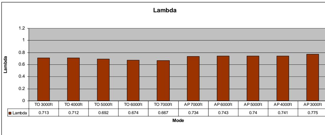
Figure 23: Change of lambda during full power climb and approach at 45% engine load. All measurements with mixture “full rich”. Lambda decreases with increasing aircraft height. The air/fuel mixture gets richer the higher the aircraft flies. At approach power, the mixture is less rich than at climb full power. (ECERT 8)
