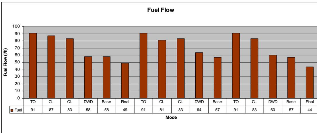
Figure 72: Fuel flow during three aerodrome circuits (TO = Take off roll, CL = Climb at v<sub>y</sub>, DWD = downwind). No “Final” measurement at the second circuit. (ECERT 56, HBKIA)
