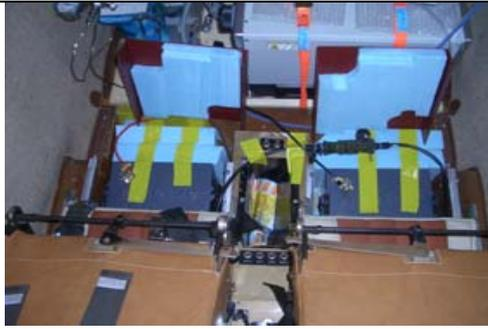
Installation of both batteries underneath the front seats. They are fitting perfectly in the place and can't slide. The lids protecting the batteries' contacts are open on the photo.
