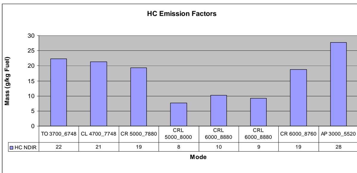
Figure 2: HC emission factors for take-off, climb, cruise and approach. TO, CL, CR5000\_7748, CR6000\_8760 and AP have been flown with air-fuel mixture “full rich”. CRL has been flown with manually adjusted air-fuel mixture.
