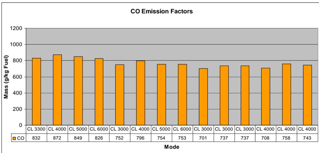
Figure 94: CO emission factors for AFM<sup>9</sup> climb power, measured at different flight altitudes, e.g. CL 3300 means climb measurement at 3300ft pressure altitude (From left to right: No 1 – 7 from ECERT58, No 8 – 11 from ECERT61 and No 12 – 17 from ECERT 65).
