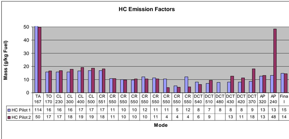
Figure 109: HC emission factors comparison for both flights. TA = taxi, TO = take-off roll, CL = climb, CR = cruise, DCT = descent, AP = approach. The number below the flight mode indicates flight pressure altitude, e.g. DCT 5100 = measurement during descent at 5100ft. (ECERT 57 and 64)
