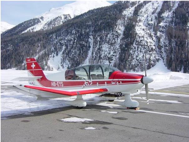
At this high altitude airport, the engine air/fuel mixture should be adjusted to less rich conditions already prior to take-off. We wanted to compare the resulting emission factors when the mixture was adjusted on ground and not during flight, as we had done in the simulated circuits at 6000ft (figures 6, 9, 12 and 15).
