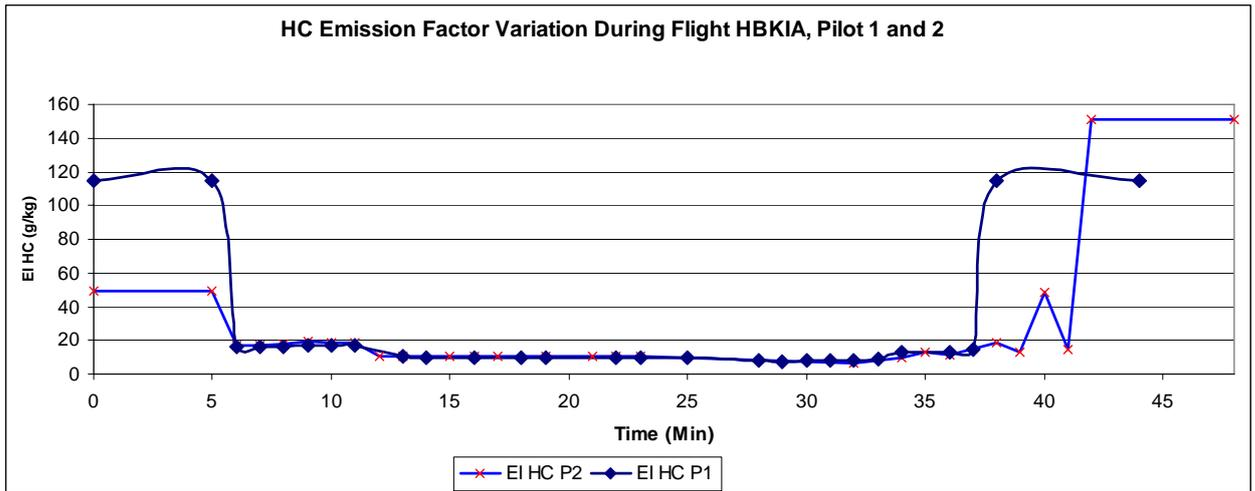
Figure 123: Comparison of HC emission factor variation during flights with pilot 1 and 2. The much higher HC emission factor during taxi (pilot 1) can be explained by lower engine RPM. At low engine RPM, EI HC drastically increases with decreasing engine RPM.
