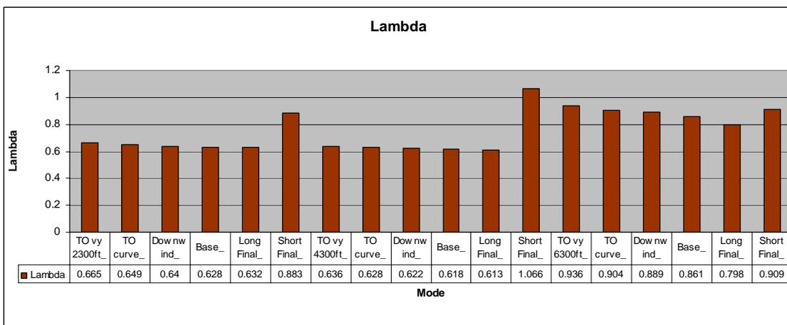
Figure 43: Lambda values in three simulated circuits, starting at 2300ft, 4300ft and 6300ft. The first two circuits were flown with air/fuel mixture “full rich”, the circuit above 6300ft with leaned mixture (right hand side). This engine shows even richer combustion (lower lambda) than that of HBEYS at “full rich” setting. (ECERT22, HBKEZ)
