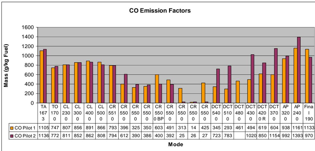
Figure 108: CO emission factors comparison for both flights. TA = taxi, TO = take-off roll, CL = climb, CR = cruise, DCT = descent, AP = approach. The number below the flight mode indicates flight pressure altitude, e.g. DCT 5100 = measurement during descent at 5100ft. (ECERT 57 and 64)
