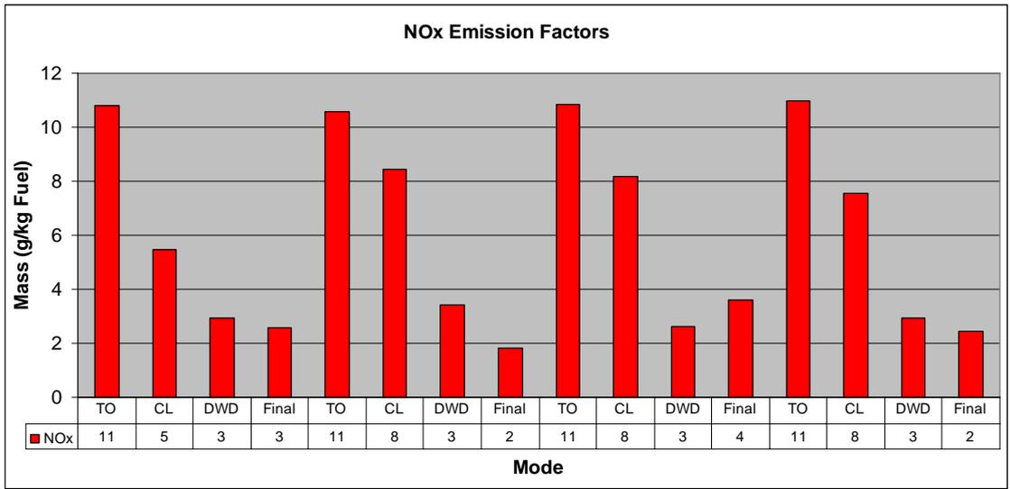
Figure 77: NO<sub>x</sub> emission factors during four aerodrome circuits (TO = Take off roll, CL = Climb at v<sub>y</sub>, DWD = downwind), flown with second pilot (ECERT 62, HBKIA)
