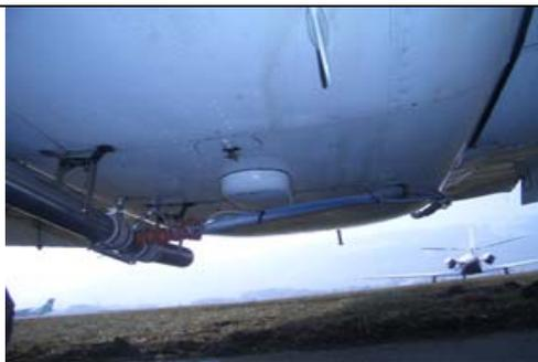
Collector pipe is directly fixed to the fuselage by choke collars.
